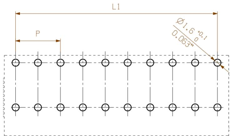
For the mounting of PCBs, it should be noted that the rated data relates only to the PCB components alone. The necessary creepage and clearance paths must be observed in connection with the respective applicant in accordance to IEC 664 / VDE 0110. The current-carrying capacity and pitch tolerance is to be determined according to DIN IEC 326 part 3 very fine.
