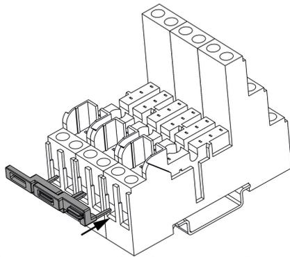
Plug the cross connection into wire-connection opening
