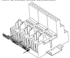
Plug the cross connection into wire-connection opening and fix it with tighten the screw
