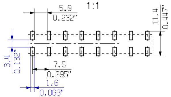
For the mounting on PCBs, it should be noted that the rated data relates only to the PCB components alone. The necessary creepage and clearance paths must be observed in the relevant equipment standards in accordance with IEC 664 / VDE 0110. The current-carrying capacity and pitch tolerance is to be determined according to DIN IEC 326 part 3.
