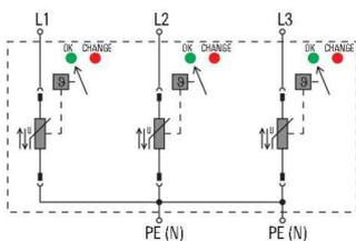
Schematic circuit diagram
