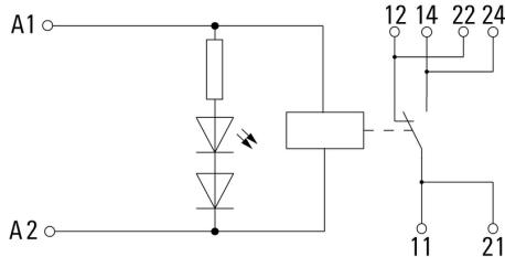
For full continuous current (16 A), the wire terminals 11 with 21, 12 with 22 and 14 with 24 must be bridged with a wire  $\geq 1,5 \text{ mm}^2$  at the socket.
