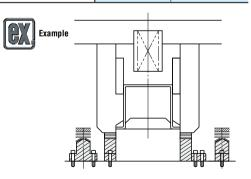
Used to cut scrap from the ring during trimming.
